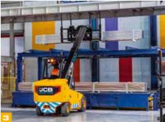
The electric Teletruk is designed to deliver greater operational efficiency inside the warehouse by supporting the continuous operation of other materials handling machines.
